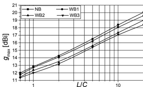
Fig. 3. Maximal antenna gain versus normalized antenna length.
